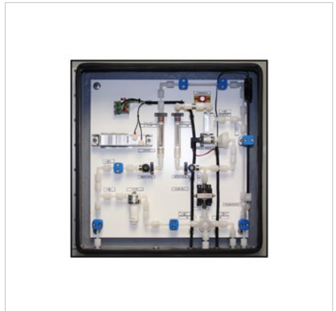
Teflon system for Cl 2 and NCl 3 (both steel-corroding)
