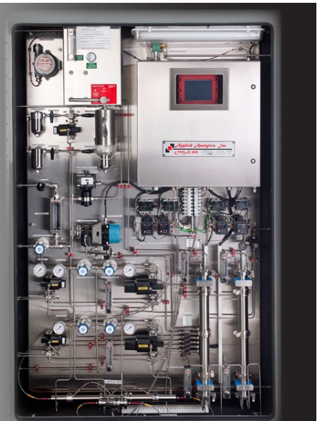
Double Headspace for \text{H}_2\text{S} and \text{NH}_3 in water
