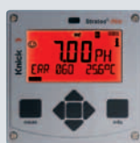
Red blinking: Alarm, error
