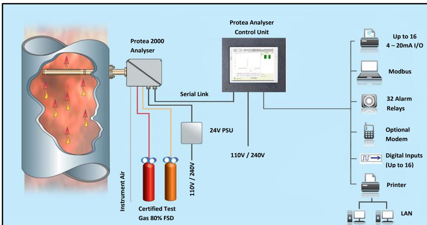
**Analysers:** The Protea 2000 analyser operates on the proven, single beam, dual-wavelength IR principle. Mid IR Pulses, at two specific wavelengths per monitored component, are transmitted through the sample cell. The 'measure' pulse is partially absorbed by the gases being measured while the 'reference' pulse remains unaffected. Up to eight wavelengths are available, sometimes sharing reference wavelengths, allowing up to six gas-phase component concentrations to be monitored simultaneously.
