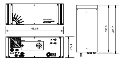
Solus is a stand-alone gas monitoring unit designed for precise measurements of single component gases. Protea has a successful history in pioneering the use of full-spectrum FTIR analysers for process and emissions gas measurements in the UK. Using our experience of analyser design and knowledge of customer requirements, Solus has been developed to give selective gas measurements in a cost-effective and efficiently packaged design.
