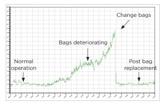
Figure 2: PCME LEAK ALERT 73 monitoring bag-leak conditions
