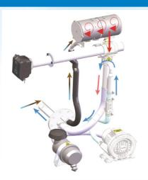
The QAL 182 WS utilises direct extractive heated sampling which can be configured to either extract an isokinetic sample or extract a sample based on a pre-set user-defined velocity. The extracted sample passes directly into a heated vaporising chamber. The sample is superheated and exits into a controlled sample chamber. The *ProScatter*\* sensor provides a high accuracy, high resolution measurement meeting ELV's of 15mg/m³ or less.
