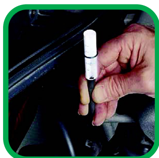
FLOW METER QUICKLY INDICATES PRESENCE OF SEALANT
