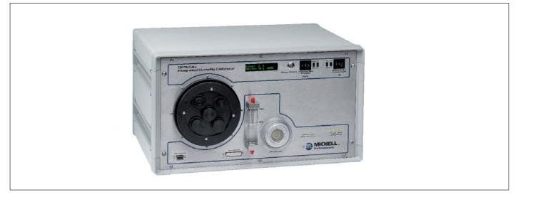
The OptiCal is a premium calibration solution for humidity sensors. The stand-alone and transportable calibrator requires no external services other than mains power, and features an integrated chilled mirror reference instrument to enable the operator to perform calibrations that are traceable to national standards.
