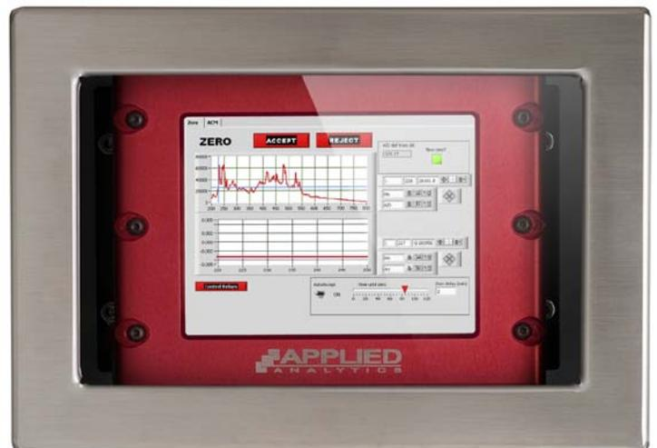
Auto Zero: Runs on custom schedule to normalize the spectrophotometer readings on zero-absorbance fluid.
