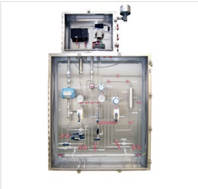
H 2 S sampling system for offshore platform environment (super duplex stainless steel enclosure for withstanding maritime punishment)
