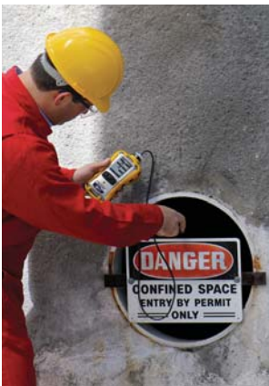
Confined space testing with the MultiRAE Lite
